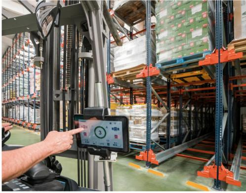
The operators place the motorised shuttle into the right channel, deposit the pallets in the first position of the racks, and then the Pallet Shuttle autonomously transfers these directly to the first free location. The reverse operation is performed to remove the goods.
