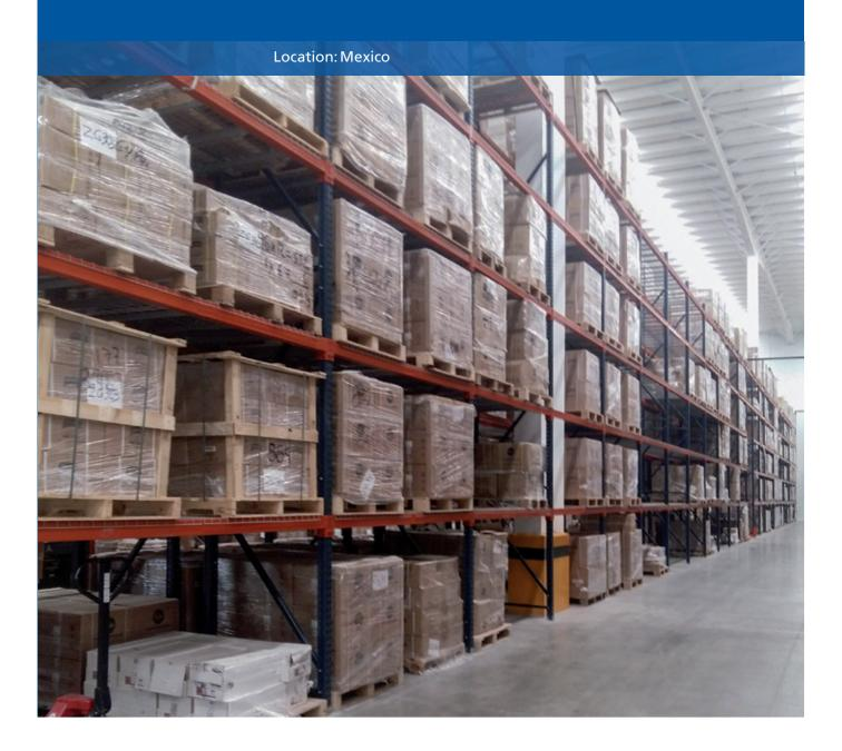
Mecalux has equipped the new ASSA ABLOY warehouse, the intelligent lock and security solution company, with pallet racks. This solution attains a storage capacity of more than 6,400 pallets of diverse sizes, weights and rotations.
