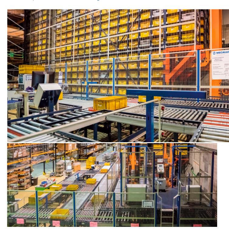
Two U-shaped picking stations are set up perpendicular to the main circuit. Picking is done via the "product-to-person" principle, in other words, the stacker cranes provide the merchandise to the operators automatically. The operators then extract the items indicated on a screen by the system and deposit them into the corresponding order.
