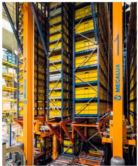
In each one of the aisles, a twin-mast miniload stacker crane circulates, whose task is to carry out the inputs and outputs of the goods automatically. These machines operate at a travel speed of 250 m/min and 90 m/min when elevated.
