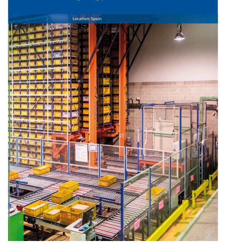
Mecalux has equipped the JCH warehouse in Barcelona (Spain) with an automated miniload warehouse that offers a storage capacity of 4,076 boxes. In addition, there is a conveyor circuit and three picking stations installed (one is also used for replenishment). The supply includes the Easy WMS warehouse management software, which ensures maximum productivity when preparing orders.
