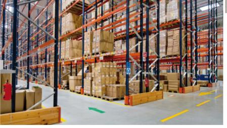
Decathlon, the established sports equipment chain, has constructed a new 30,000 m² logistics centre in Łódź (Poland) and Mecalux has fitted it out with picking shelves and pallet racks. Both solutions help classify the goods according to their dimensions and demand, while also providing direct access to speed up order picking, this centre's primary operation.
