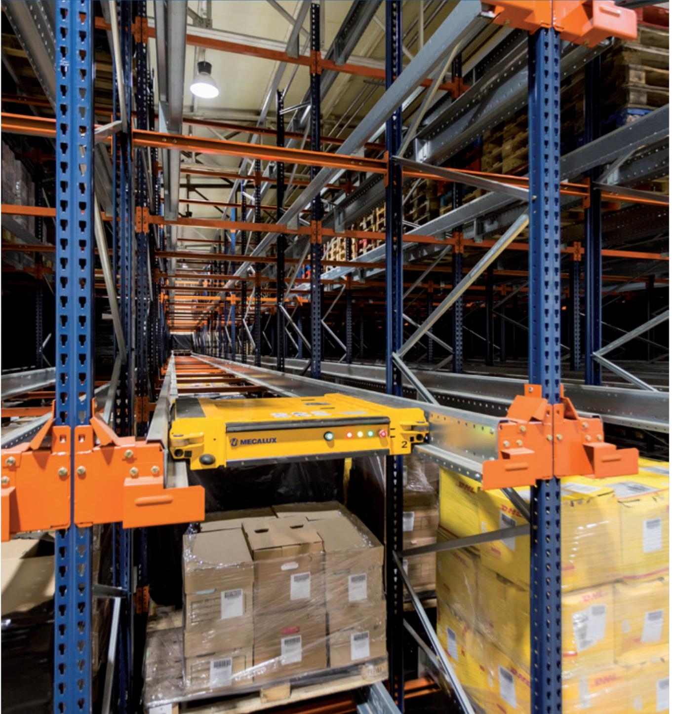
Optimising the space of a warehouse is essential if you want to achieve a high storing capacity. Mindful of this issue, nr docusafe has installed high-density pallet racks operated by an automatic shuttle of Mecalux in its documentary vault at Senningerberg (Luxembourg).
