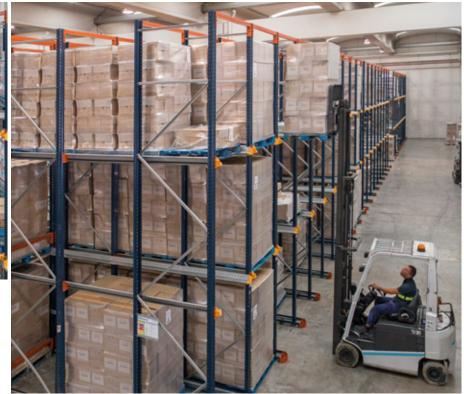
Each lane level has support rails on both sides. Made in a compact triangular-shape, these facilitate the placement and support of the pallets
