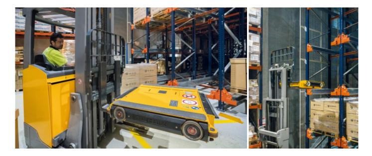
This sequence is repeated as many times as needed. The same process is carried out in reverse from the opposite side of the block of racks to remove the goods.
