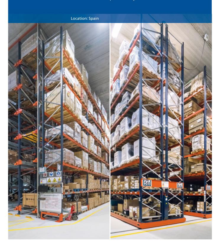
EGO Appliance Controls obtained a solution tailored to its needs in the warehouse it owns in Lliçà de Vall (Barcelona). Mecalux equipped the facility with the high-density Pallet Shuttle system, two blocks of Movirack mobile racks and pallet racking.
