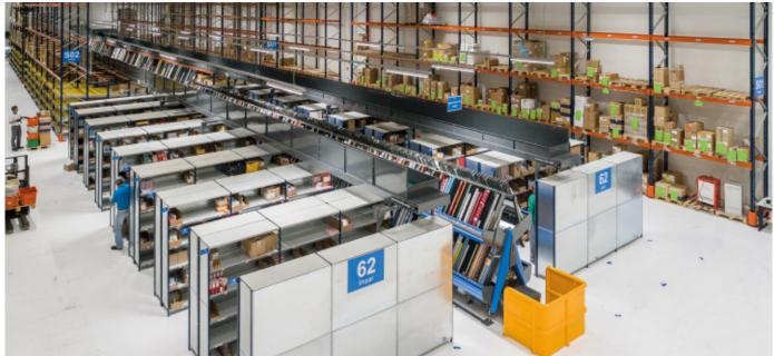
Operators remove items from the inside of the first box and place them in the corresponding carton compartment from the automatic box dispenser. The advantage of this storage system is stock reserves are housed on the same level, behind the first box, meaning the product is always there for the taking.
