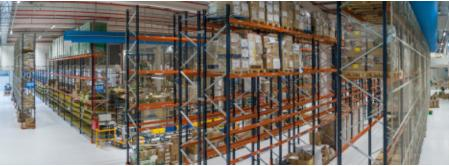
In the other two, dedicated to type B and C products, live storage for picking was installed with two attached conveyors and light-duty shelving units for the lower consumption boxes.
