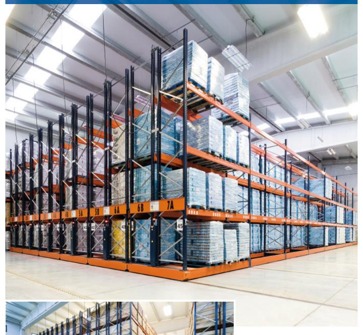
Mecalux has equipped the Connorsa warehouse, one of the most renown canned food producers in Spain, with pallet racking and two blocks of Movirack mobile pallet racking. With this solution, the company procures a storage capacity for 8,600 pallets, organised according to their characteristics and demand.
