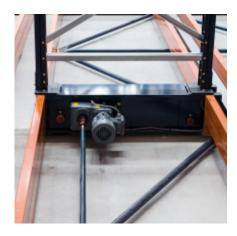
The transmission of power to the mobile base is undertaken through a double crown gear with a double pinion, which provides better system performance. By doing so, this ensures that the movement of the racks is more uniform and, therefore, the life of the mechanical components is extended.
