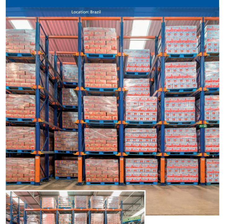
The Lacticínios Bela Vista company has purchased three different storage systems from Mecalux for its distribution centre in Minas Gerais (Brazil): drive-in pallet racking, pallet racking and live storage racks. The installation has a storage capacity of 6,320 pallets, the best fit to meet the expected growth rate.
