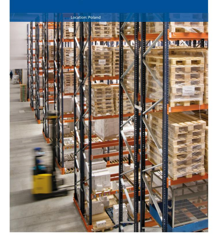
Ziaja, Polish manufacturer of natural cosmetics and pharmaceuticals, has a new warehouse designed specifically to streamline picking, the chief operation of the centre. Mecalux has installed standard pallet racking, which offers direct access to the goods and has a storage capacity of 10,906 pallets.
