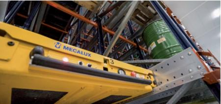
Serfrial, a logistics operations company within the Grupo Fuentes, has renovated two of its cold stores located in the town of Las Torres de Cotillas (Murcia). The company has fitted them out with high-density racks operated by the semiautomatic Pallet Shuttle system, meaning it enjoys a total storage capacity for 26,880 pallets.
