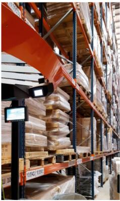
The operator views the movement and direction of the forks on a screen when handling the merchandise.
