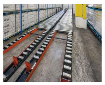
This preload system regroups pallets of the same order or route, and streamlines distribution vehicle loading
