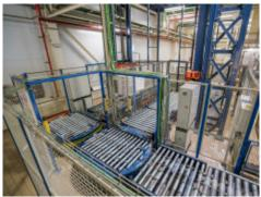
The lifts, which can shift two pallets at a time (one behind the other), are capable of absorbing outputs from production in a relatively short period of time
