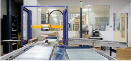
A parallelly placed, non-motorised roller conveyor lets warehouse operators move boxes manually to the handiest work position.
