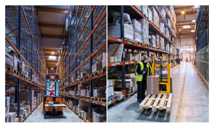
Ground level pickers are responsible for items located on the first shelf or those on the floor. Meanwhile, the high reaching order picking equipment facilitates access to the goods deposited on the second and third shelves.
