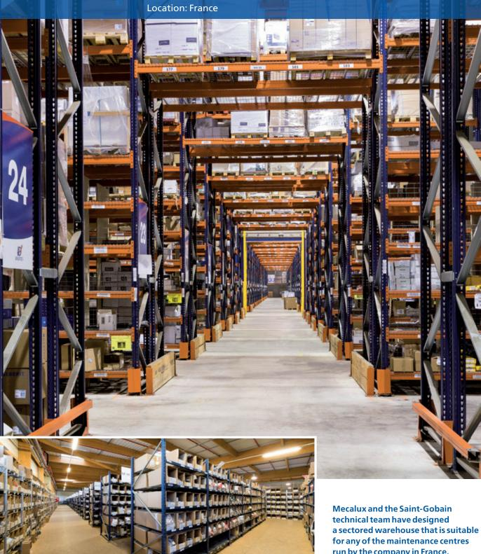
for any of the maintenance centres run by the company in France. The solution consists of combining pallet racking, cantilever racks and various picking solutions.
