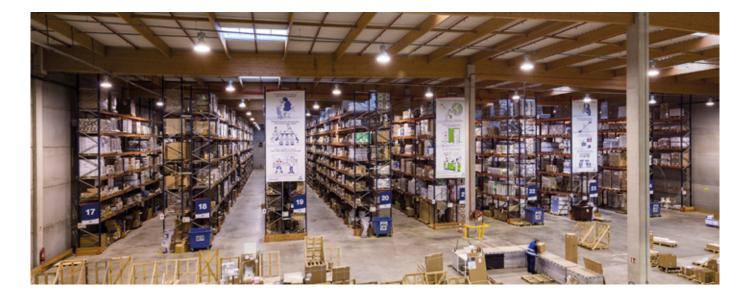
The racks are fitted out with underpasses that cut across the blocks to streamline workflows and, at the same time, to serve as emergency exits
