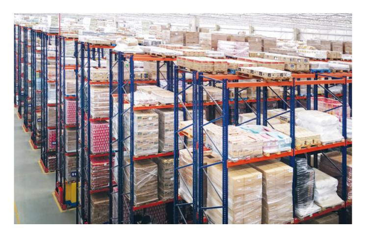
The products in greatest demand are placed at the ends of the aisles, closest to the loading bays, to speed up their movement in and out of the warehouse
