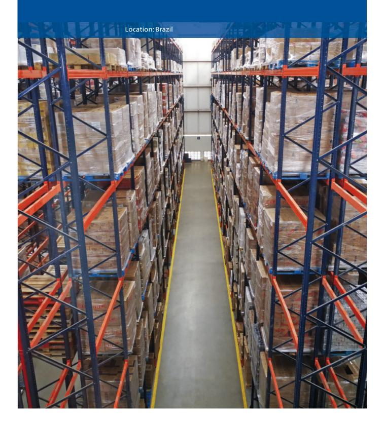
The Brazilian supermarket Super Nosso has opened a new 25,000 m<sup>2</sup> distribution centre in Contagem (in the state of Minas Gerais). Mecalux has equipped it with 15 m high pallet racks with a total storage capacity of 37,800 pallets. These offer direct access to the products, which simplifies preparing the 3,000 daily customer orders.
