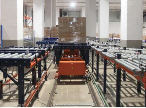
electromechanical equipment (conveyors, stacker cranes, transfer cars, etc.) carry out operations that, in a non-automated warehouse, would otherwise be done by workers operating traditional forklifts (mainly, in-house transporting and slotting of the goods in the racks).
