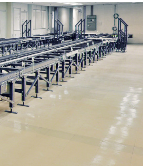
The conveyor is 48.3 m long and runs at speeds of 20 m/min
