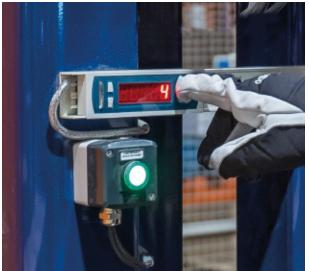
The put-to-light device shows the number of SKUs to place on each pallet. Once the process has been completed, the operator presses the button to validate their picking. This system provides high operational agility, reduces errors in order preparation and enables real-time stock updates by transmitting all information to the WMS.
