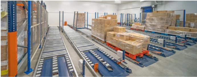
Goods kept safe. The dispatch area also works at a controlled temperature to not break the cold chain. Additionally, retainers, brake rollers and other devices installed in the preload channels automatically control pallet speeds and stops, without jamming or collisions.
