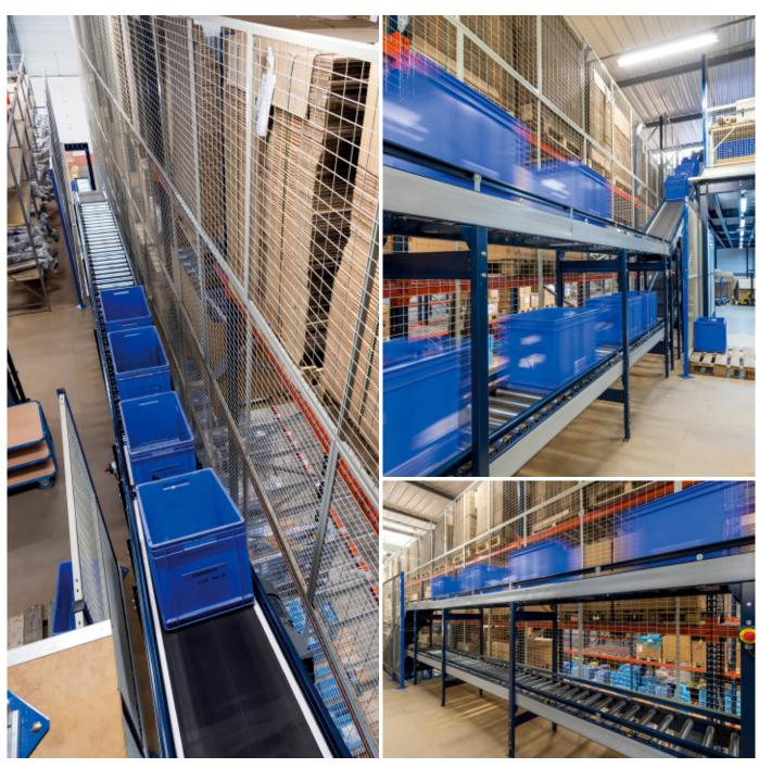
A combination of roller and belt conveyors run along the route. The inclined belts are very useful in dealing with slopes in the warehouse.
