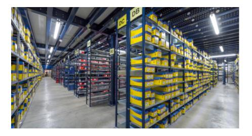
The picking shelves on the three warehouse levels provide direct access to the goods, which simplifies storage and picking tasks. Operators must only collect the items that comprise each order directly from the shelves.
