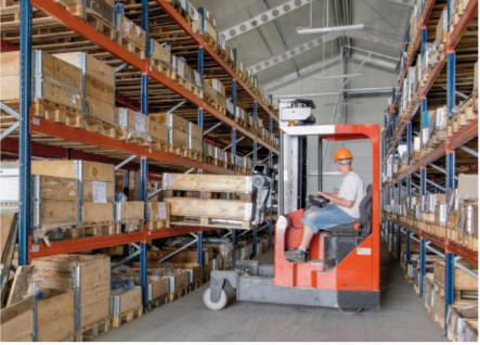
The metal profile warehouse of MetalERG comprises both pallet racks and cantilever racks. These two systems are able to accommodate different sized products with distinct features, as well as supply direct access to the goods, which translates into streamlined storage and pick tasks.
