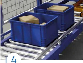
Once picking has finished, the storage tote returns to the AS/RS or is sent to another workstation. The completed order is moved to the consolidation area or directly to shipping.
