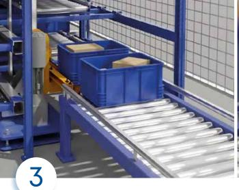
The conveyor system **transports the tote to the pick station**. There, the operator receives order fulfilment instructions from the warehouse management system.
