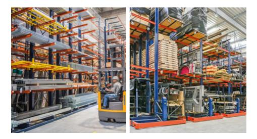
THESE RACKS CAN BE INSTALLED ON MOBILE BASES TO INCREASE STORAGE CAPACITY.
