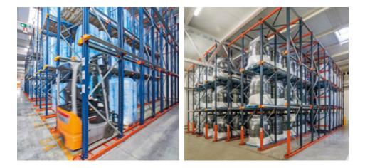
CAN BE USED WITH EITHER LIFO (LAST IN, FIRST OUT) OR FIFO (FIRST IN, FIRST OUT) WITH BATCHES WHEN THERE ARE MORE THAN THREE LANES PER SKU.
