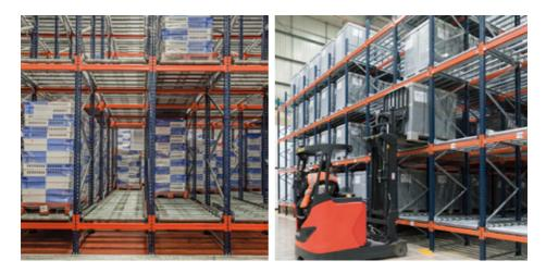
UNINTERRUPTED FLOWS: NO INTERFERENCE BETWEEN LOADING AND UNLOADING OPERATIONS BY DESIGNATING A DIFFERENT AISLE FOR EACH TASK.
