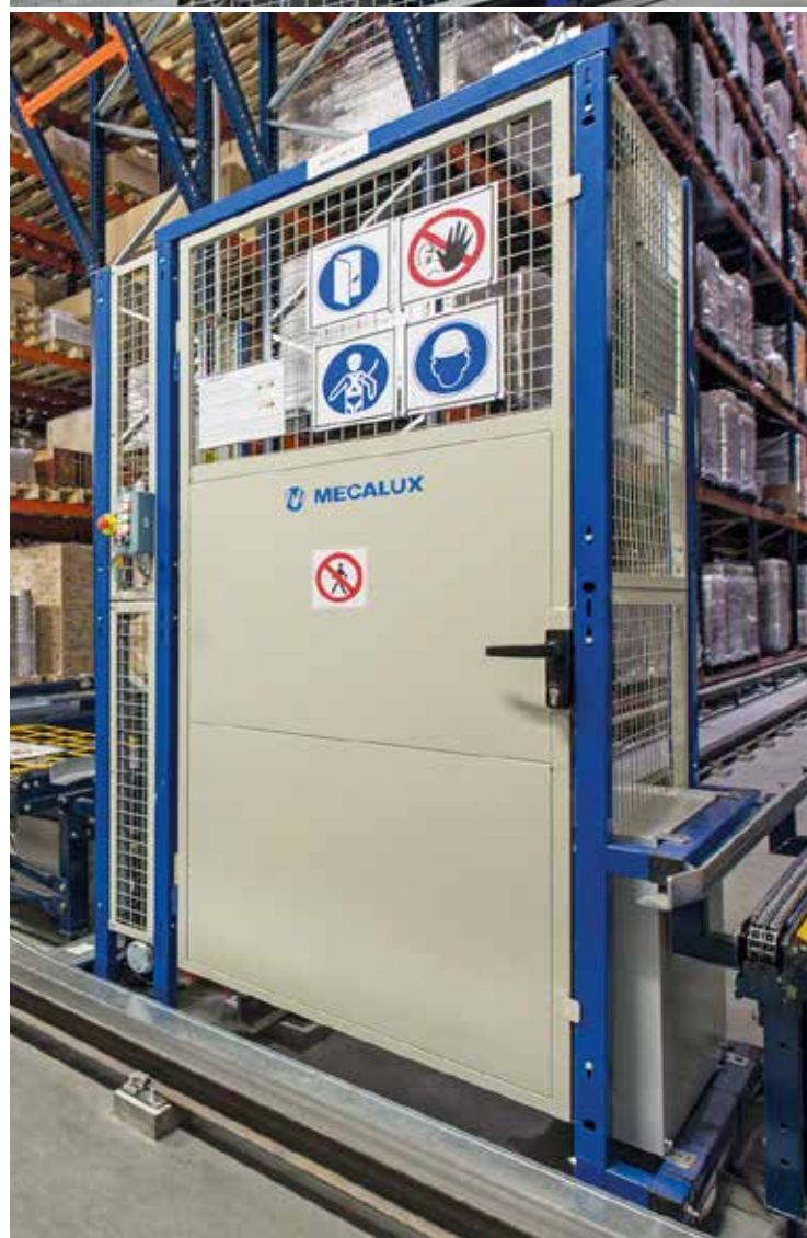
Control and maintenance zone partitions.
