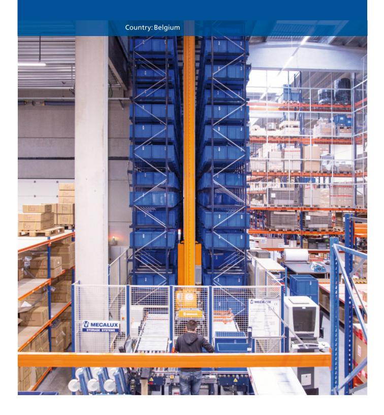
TAL, a Belgian manufacturer of high-quality lighting systems and accessories, has equipped its new distribution centre in Pittem, Belgium, with an automated warehouse for boxes. Its aim is to optimise space, ensure safe goods storage and minimise errors, ensuring the productivity required by omnichannel retail. Managed by Easy WMS, the facility holds approximately 1,400 SKUs in 6,300 boxes. Mecalux has also installed pallet and cantilever racks to store larger products.
