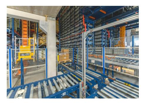
plete logistics solution comprising various AS/RS, pallet racks, and automated management, all of which has increased the number of orders prepared by 27%.
