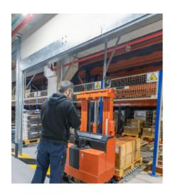
Two areas with manual live channels for boxes and pallets, also fitted with pick-to-light devices.
