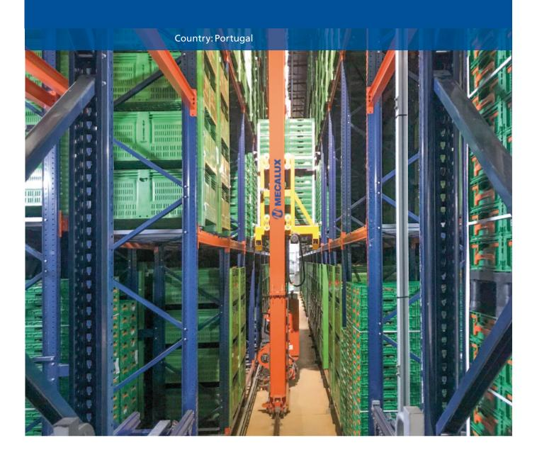
Kiwi Greensun, the Iberian Peninsula's largest producer of kiwis, has overhauled its fruit ripening room in Salvador de Briteiros, Portugal, with the construction of an automated clad-rack warehouse by Mecalux managed by Easy WMS. With this installation, the company has its sights set on raising production to 12,000 t of kiwi fruit a year. One of the advantages of this warehouse with fully automated operations is the accurate control of products stored at refrigerated temperature.
