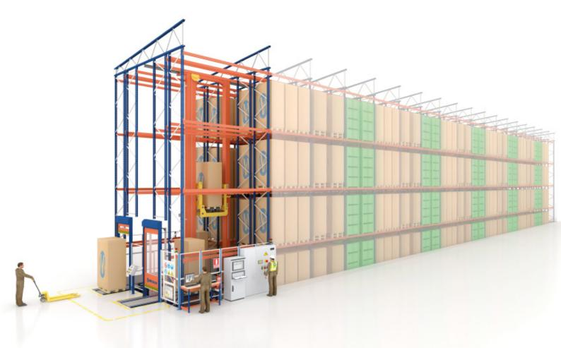
The racking, divided into four levels, has been personalised to be able to accommodate three different unit loads:  $1,200 \times 1,200 \text{ mm}$  plastic containers and pallets measuring  $800 \times 1,200 \text{ mm}$  and  $1,000 \times 1,200 \text{ mm}$ . In the case of plastic containers, each location can store up to four containers stacked one on top of the other
