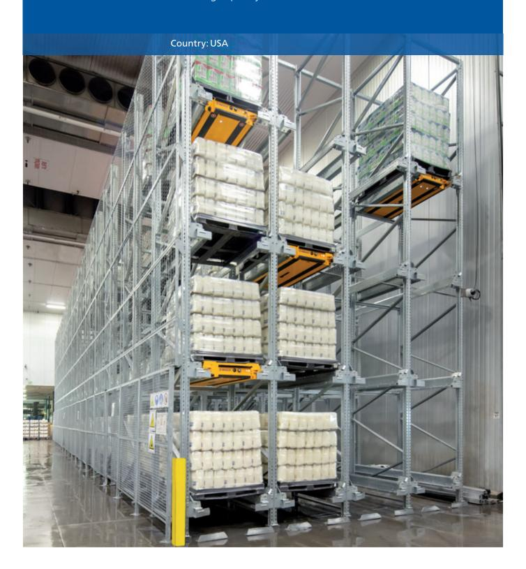
Dairy products supplier and distributor Producers Dairy recently installed a semi-automated Pallet Shuttle for its 4,645 m<sup>2</sup> cooler at its plant in Fresno, California. The Pallet Shuttle replaced the company's outdated and inoperable pallet racking system. By installing the Pallet Shuttle system, the firm was able to double its capacity and prepare 300 orders per day.
