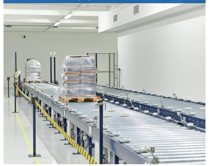
Vibar Nord, a producer of over 5,000 tonnes of food and dietary products a year, has opted for robotics in its new warehouse in Gera Lario, northern Italy. Mecalux has automated the connection between the production plant and dispatch area via a dual conveyor line and a pallet lift that automatically join the two zones. Mecalux has also implemented two earthquake-proof storage systems: Movirack mobile pallet racking and pallet racks, which have increased Vibar Nord's warehousing capacity by 70%.
