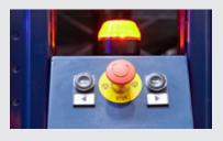
**Emergency buttons immediately** block the movement of the racks in the event of an incident.
