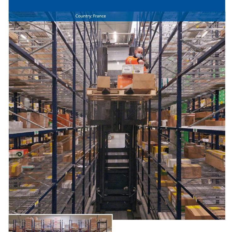
Cooperative VST has expanded its logistics centre in Les Essarts, France, and Mecalux has equipped it with Movirack mobile racking and multi-tier picking shelves. They have capacity for over 13,000 containers, which are stored according to their physical characteristics and weight. With this combination of solutions, VST has optimised its available space, sped up order preparation and reached its goal to dispatch more than 200 orders a day.
