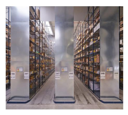
tre in Les Essarts. This facility serves the 750 members that form part of the cooperative. With the installation of two storage systems in one space, the company has achieved its goal. Movirack mobile racking is the only compact system that provides direct access to the goods in addition to optimising the surface area
