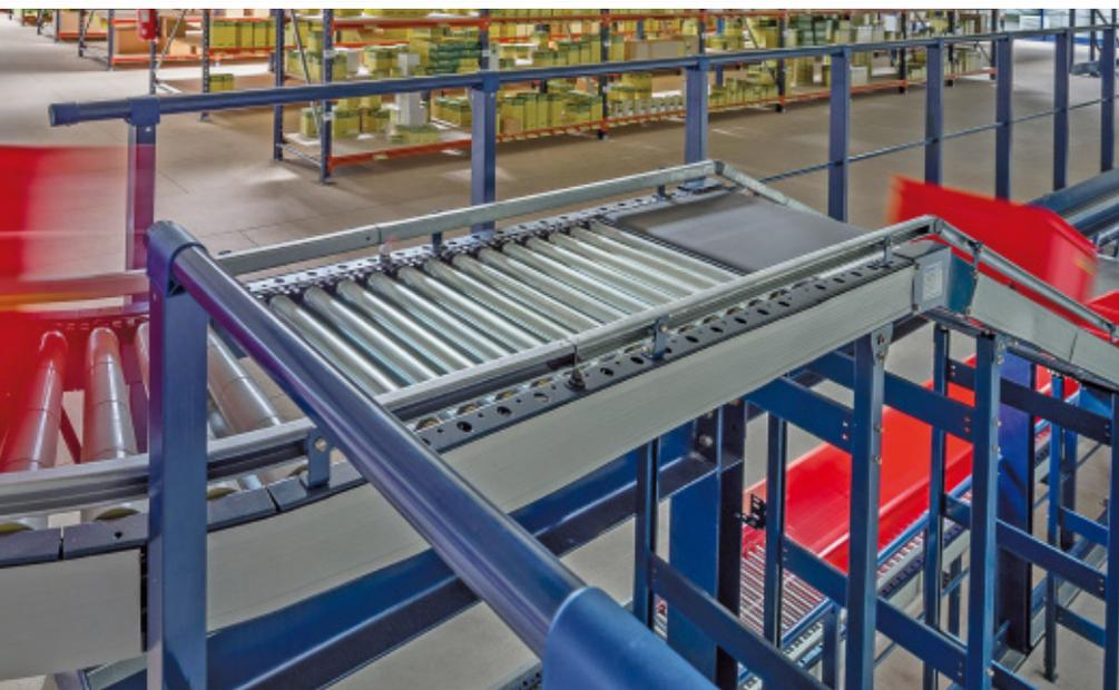
The conveyor belts allow height differences to be overcome and movements to be carried out at different levels, while the swing conveyors allow the passage of the operators
