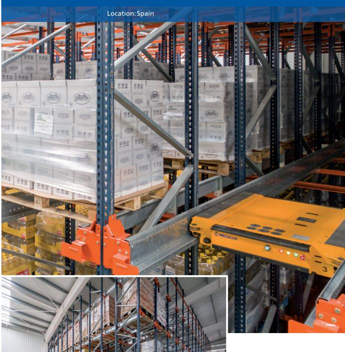
Mecalux has set up two blocks of racks that run with the semi-automatic Pallet Shuttle system in Aceites Toledo's distribution centre. This solution, designed especially to store bottled product, provides a storage capacity for 1,880 pallets and streamlines incoming and outgoing goods from the respective channels.
