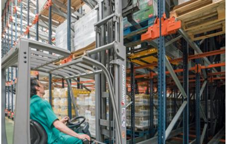
The high-density Pallet Shuttle system at Aceites Toledo holds more than 1,880 pallets allocated throughout 136 storage channels
