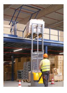
This installation houses Puccini's vast product range. Taking into account the limited space and type of goods to be stored, the company decided to instal a mezzanine floor that would double the useful storage area. To manage the goods, Mecalux fitted out the mezzanine floor with M7 heavy-duty shelving.
