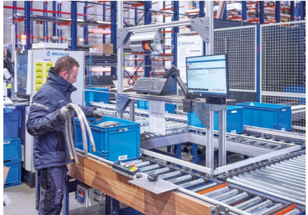
to the goods-to-person method. These operators remain at their workstations as the products are brought to them. They then sort the items in the carton live storage located behind them. This system stands 2.2 m tall and is made up of slightly inclined roller platforms. Hence, once an order is closed, it slides by gravity to the dispatch area on the opposite side.
