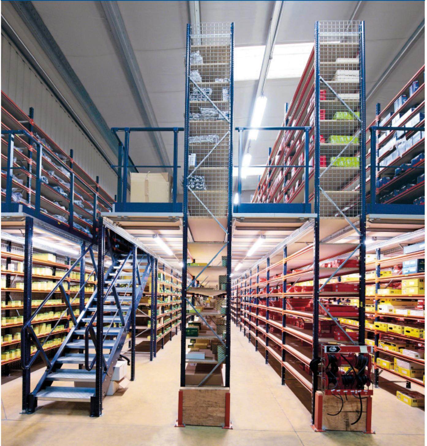
Eagle Spare Parts has a 2,400 m<sup>2</sup> warehousing facility in the town of Mours-Saint-Eusèbe (France) equipped with Mecalux shelves with walkways. These shelves help to classify goods according to their dimensions and demand level, while providing agility in storage tasks and order fulfilment processes.
