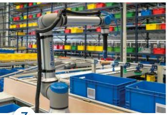
**Product picking and placing**. Using the data provided by the Siemens vision software, the robotic arm picks the selected product and places it in the corresponding order tote.
