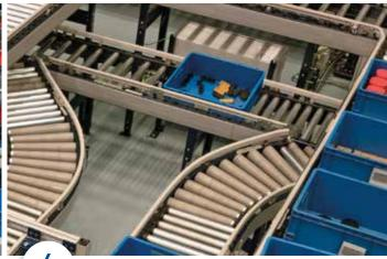
**Picked order.** Once picking has finished, conveyors transport the tote containing the order to another area in the facility (consolidation, dispatch, etc.).
