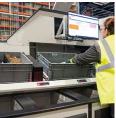
PICK-TO-LIGHT SYSTEMS STREAMLINE ORDER PICKING AND AVOID ERRORS DUE TO MANUAL HANDLING.
