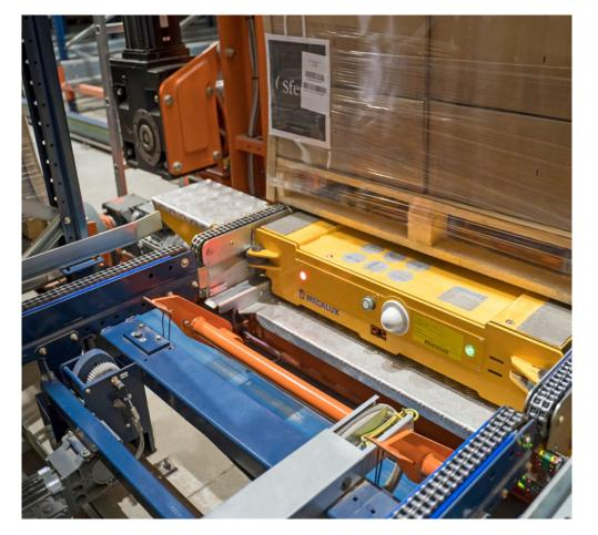
4,990 pallets with a maximum unit weight of 600 kg. The stacker crane picks up the pallets and brings them to the corresponding storage channel. An electric shuttle then moves them to the deepest available location in the channel.
