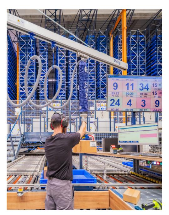
bins are subsequently placed onto a conveyor system, which transports them to the automated warehouse. A lift bridges the difference in height between the two facilities.
