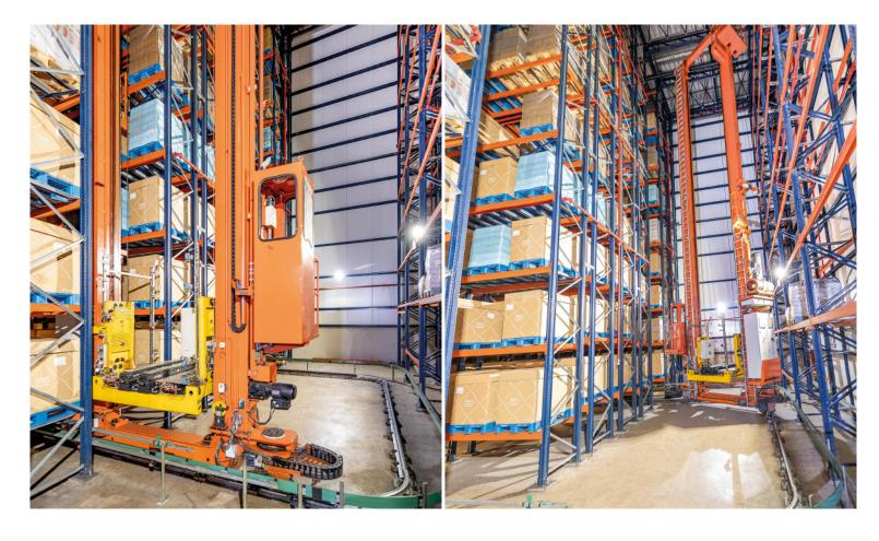
crane, which operated in the three aisles. It did so by means of a system of curved rails set up at the back of the warehouse, enabling the stacker crane to change aisles as required. This solution is implemented when the storage volume is high and the flow of movements is moderate.
