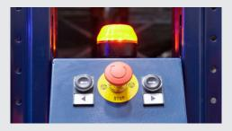
**Emergency buttons immediately** block the movement of the racks in the event of an incident.
