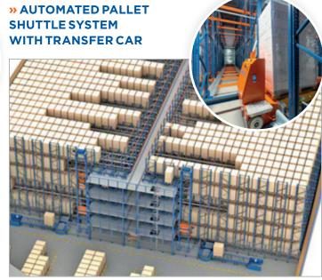
The stacker crane executes movements from the AS/RS input and output positions to any storage channel. The pallet shuttle is tasked with moving pallets from the cradle of the stacker crane to the location in the corresponding channel. Generally, two compact storage racking units are installed, one on each side of the working aisle.
