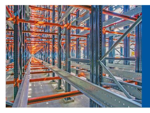
The automated Pallet Shuttle is a compact storage system that uses electric shuttles and automated handling equipment (stacker cranes or transfer cars) to boost the capacity and productivity of the warehouse. The system executes the orders given by the Easy WMS warehouse management software.
