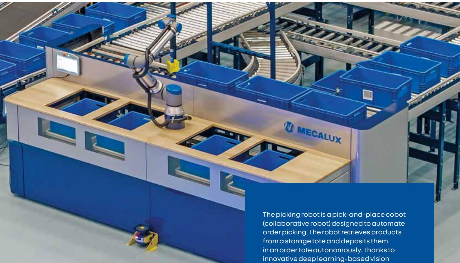
The picking robot is a pick-and-place cobot (collaborative robot) designed to automate order picking. The robot retrieves products from a storage tote and deposits them in an order tote autonomously. Thanks to innovative deep learning-based vision software and a highly versatile gripping device, the robot handles a wide variety of items with absolute precision, regardless of size, shape or finish.
