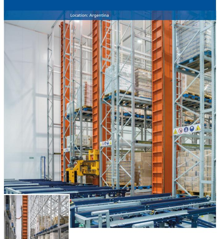
La Anónima, one of the most important supermarket chains in Argentina, has expanded its cold storage in the town of Ituzaingo (Buenos Aires), gaining greater storage capacity. Mecalux has installed an automated warehouse composed of four single-depth aisles served by trilateral stacker cranes and a conveyor circuit at the front; all managed by the warehouse management software the Easy WMS by Mecalux. This solution is designed to meet growing demand, adapting to future prospects.
