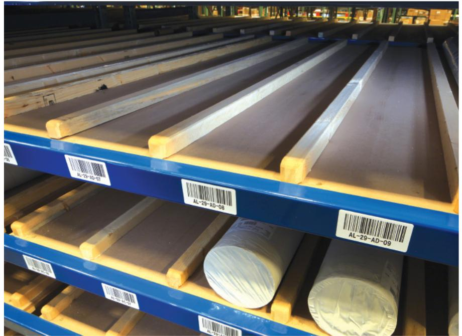
Rectangular, wooden laths serve to present shelves from bending and separate the fabric rolls stored in the racks
