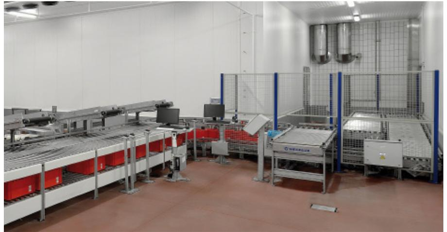
The products are previously placed in plastic boxes of the eurobox type, measuring 600 x 400 x 300 mm, forming a transport and storage unit
