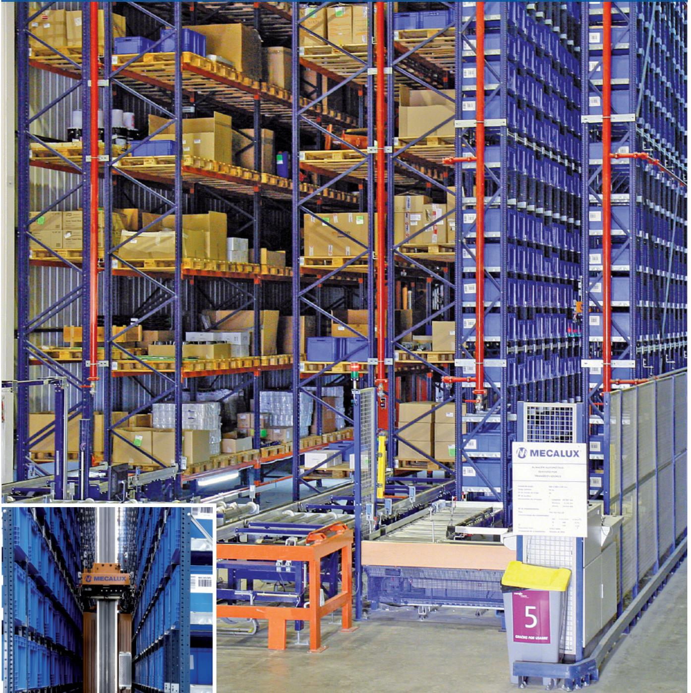
Mecalux, Renfe's regular outfitter, has designed a warehouse that is viable for any of the railway company's maintenance centres. The solution was to combine a miniload warehouse for boxes, an automated pallet racking warehouse and a warehouse with cantilever racking allocated to bulky items. Everything is controlled by the Mecalux Easy WMS warehouse management system.
