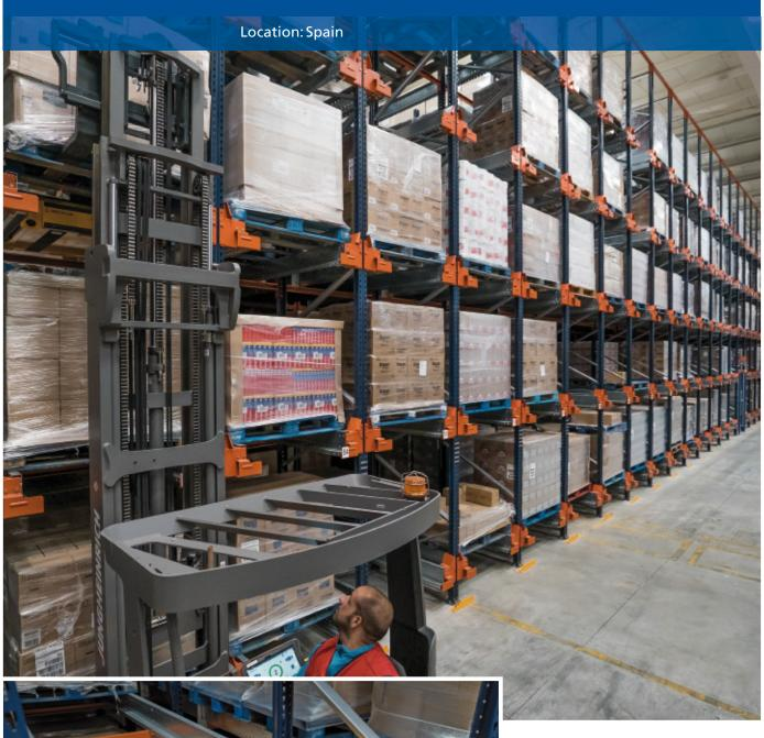
Mecalux has installed the Pallet Shuttle system in the warehouse Marvimundo has in Murcia to increase the storage capacity by more than 1,000 pallets in the same surface area and space available. That way the company maintains its commitment to innovation and constant improvement in its production processes to cope with the growth achieved in recent years.
