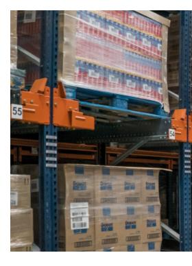
277 channels, each 6 m deep, offer a storage capacity of over 1,900 pallets (1,000 more than the standard pallet system)
